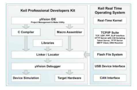
The **Keil ARTX-ARM Advanced RTOS** for ARM-based Microcontrollers is a flexible Real-Time Operating System that includes a Flash File System and TCP/IP Networking support.
